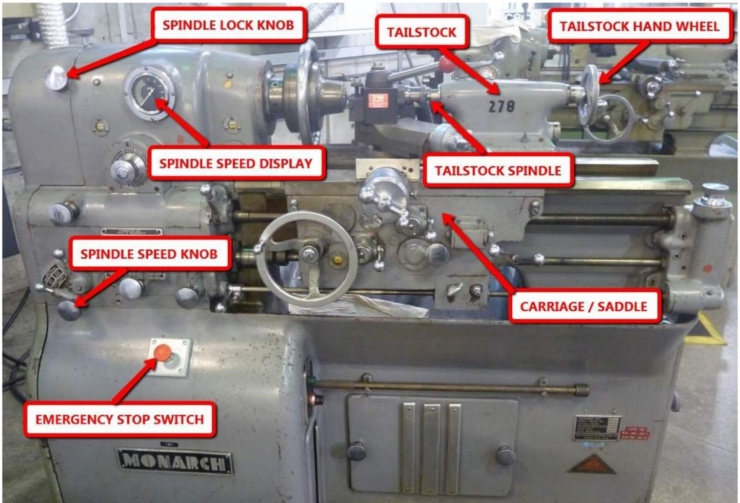
**SPINDLE LOCK KNOB** For keeping the spindle from rotation when tightening or loosening collets.
