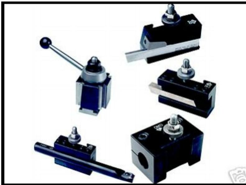
For safe and efficient cutting, the tip of the tool must be located directly on the center of the part in the chuck! Too high and the base of the tool will push on the part. This may damage your workpiece or break the cutting tool. If the tool is set too low, the tip of the tool will tend to gouge and/or cut too deep. It will also leave an undesirable “nub” when you reach the center of the workpiece.
