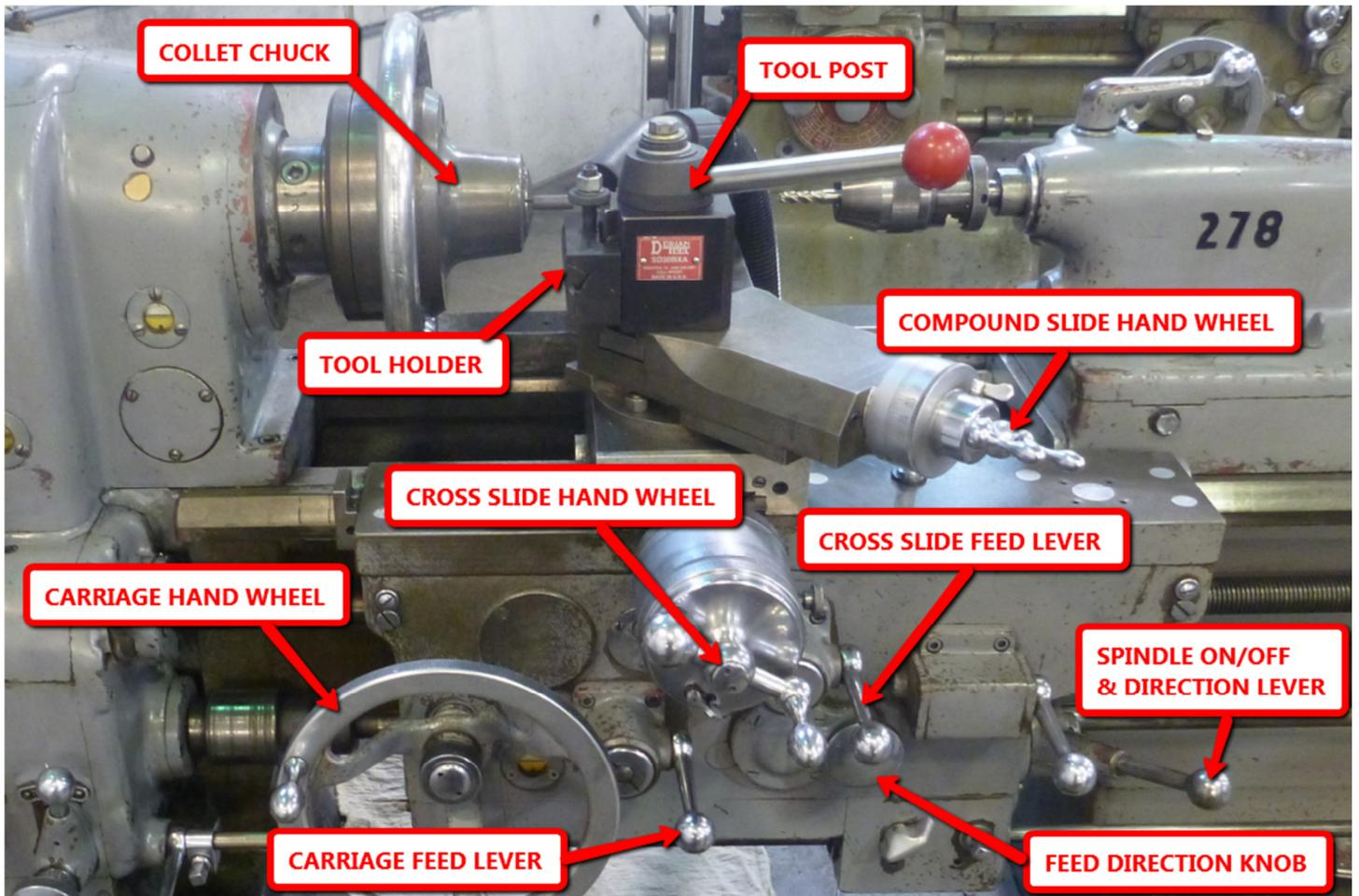
**COLLET CHUCK** For holding small diameter work pieces in the spindle of the lathe.
