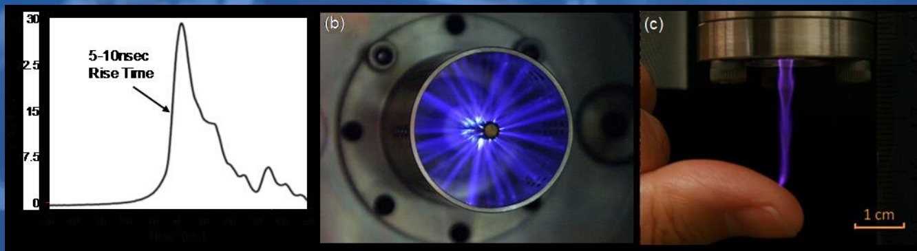
FIGURE 1. (A) TYPICAL OUTPUT CHARACTERISTICS OF NANOSECOND HIGH VOLTAGE PULSE GENERATOR. (B,C) PHOTOGRAPHS OF THE TRANSIENT PLASMA (HOT ELECTRON, LOW-TEMPERATURE PLASMA) FORMED BY THE HIGH VOLTAGE NANOSECOND PULSE APPROACH.
