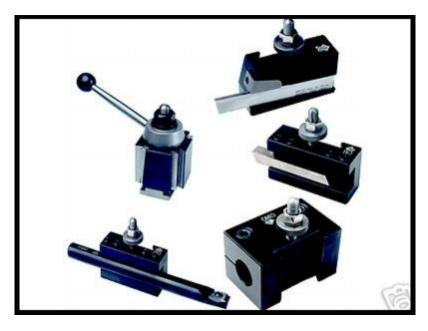
For safe and efficient cutting, the tip of the tool must be located directly on the center of the part in the chuck! Too high and the base of the tool will push on the part. This may damage your workpiece or break the cutting tool. If the tool is set too low, the tip of the tool will tend to gouge and/or cut too deep. It will also leave an undesirable "nub" when you reach the center of the workpiece.
