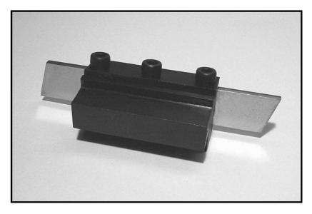
• THE CUT OFF TOOL This tool (shown above) is also called a "parting tool." It is primarily used for cutting off (aka, parting) the workpiece and making outside grooves. This tool can only cut "across" the part in one direction (along the X axis).
