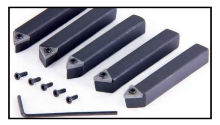
• THE LATHE BIT The image above shows the most common lathe cutting tools, they are called lathe bits. These can cut outside surfaces and edges. There are versions that consist of a piece of carbide brazed onto a rectangular steel bar. The ones in the above image are called "insert lathe tools." It is because they have a carbide insert that can be replaced or rotated when they become dull. This is ideal for those that have little or no experience in grinding their own tools.
